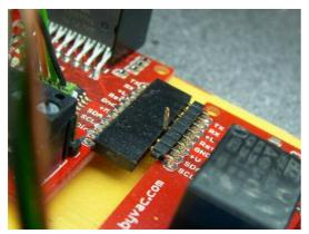
In this example, a relay is stacked to a motor controller. The supply to the motor controller is 12V through the +V pin and so as can be seen the relay is stacked because it shares all of the other pins but the +V pin is bent out of the way so that it can be connected to a separate 5V supply.
