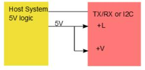
Example when connecting to a host system that uses a 5V logic supply.
