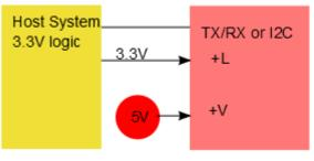
Example when connecting to a system with 3.3V logic supply
